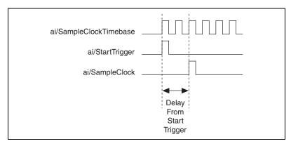
Figure 4-11. ai/SampleClock and ai/StartTrigger
